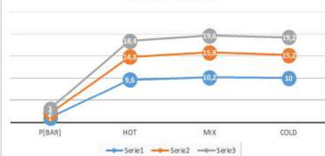
FLOW RATE [L/MIN]-G3/4" FREE DISCHARGE
