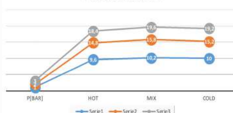
FLOW RATE [L/MIN]-G3/4" FREE DISCHARGE
