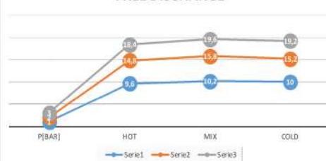
FLOW RATE [L/MIN]-G3/4" FREE DISCHARGE
